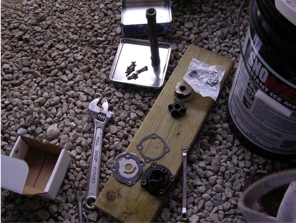
7. Below is a picture of the old pump notice the blades. This should have been replaced a long time ago!
