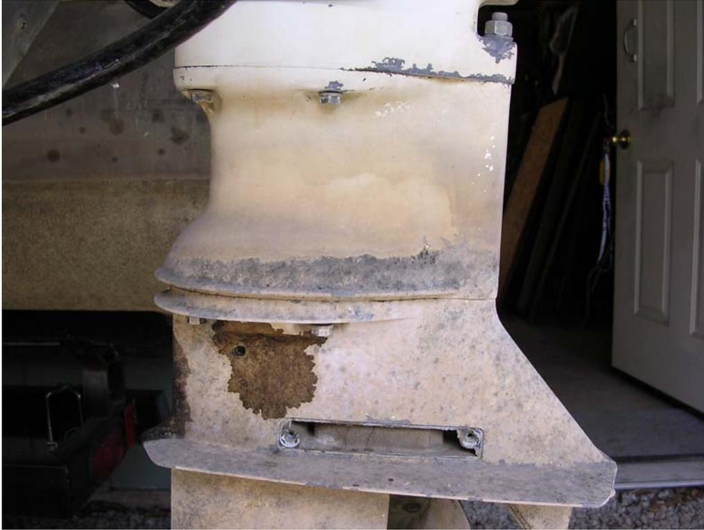
3. Now that you have the bolts loose you need to disconnect the shifting rod. On some outboards you disconnect the shifting rod underneath the block...on this motor which is a 28HP Johnson you have an access door. Note: This style is a pain in the butt in my humble opinion.....see below.
