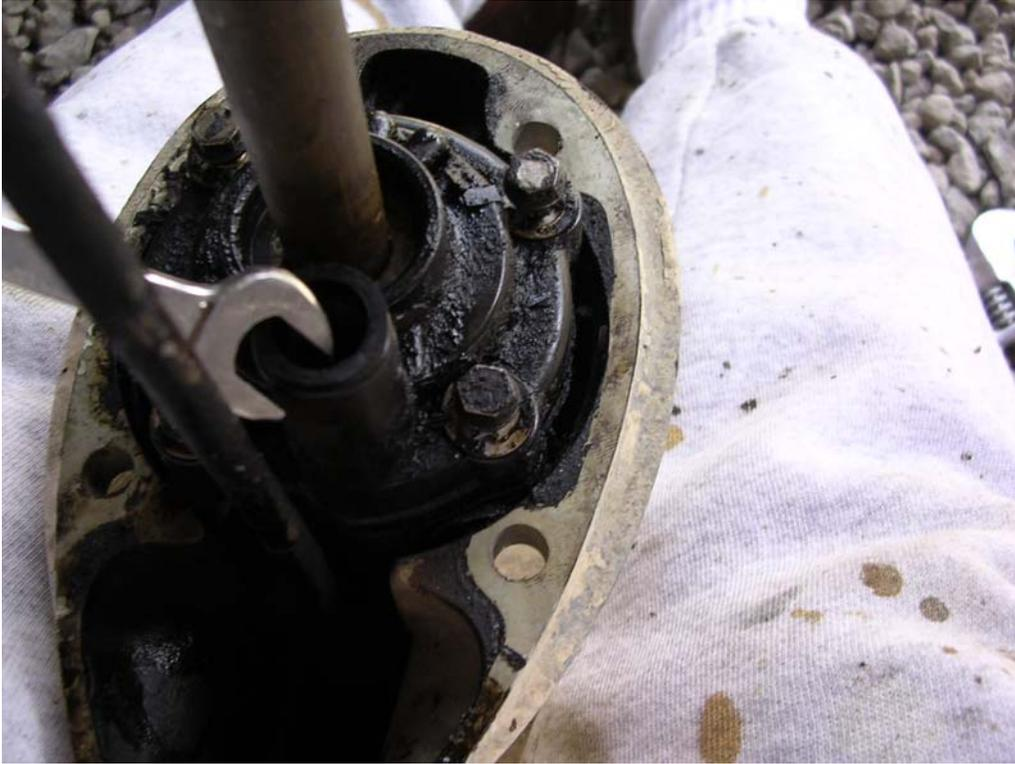
5. Again you'll want to mark everything! The next step is to replace the water pump itself. You'll need to loosen the 4 bolts as seen in the above picture. What the wrench is pointing to is where the water tube has to go when you put everything back together. This HAS to be aligned!
